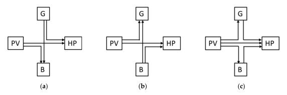
Figure 3. Schematic of the DC-bus operating in (a) charging, (b) discharging and (c) buffer modes.
