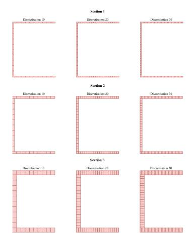
Figure 2. Selected C-shaped sections and their discretisation.
