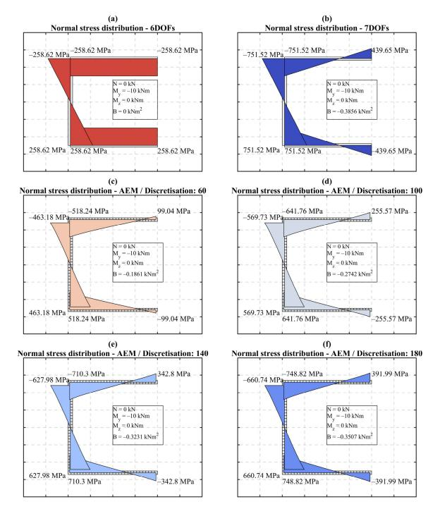
**Figure 8.** Normal stress distribution for Section #2, with a length L = 1000 mm and a section discretisation of 30 blocks for each section part.
