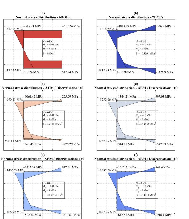
**Figure 7.** Normal stress distribution for Section #1, with a length L = 1000 mm and a section discretisation of 30 blocks for each section part.
