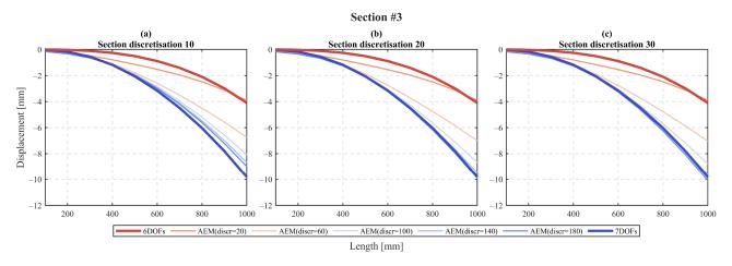
Figure 6. Vertical displacement-length relation for Section #3 with the different discretisation configurations.
