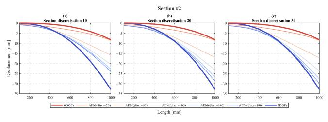
Figure 5. Vertical displacement-length relation for Section #2 with the different discretisation configurations.
