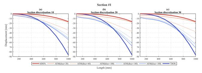
Figure 4. Vertical displacement-length relation for Section #1 with the different discretisation configurations.
