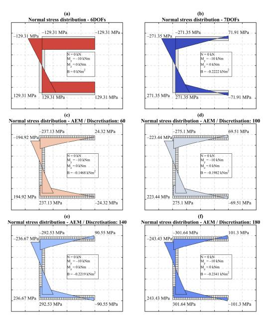
**Figure 9.** Normal stress distribution for Section #3, with a length L = 1000 mm and a section discretisation of 30 blocks for each section part.
