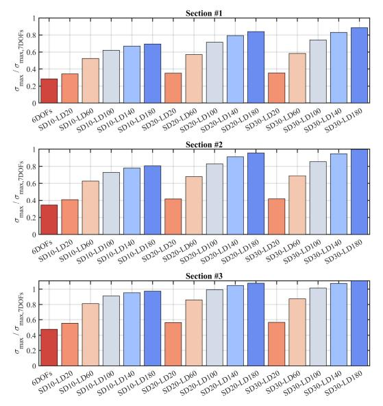
**Figure 10.** Distribution of the normalised stress peaks to stress peaks based on the 7DOFs formulation. The results correspond to the case with a length of 1000 mm, varying, in the case of AEM, the section discretisation (SD10, SD20 and SD30) and longitudinal discretisation (LD20, LD60, LD100, LD140 and LD180).
