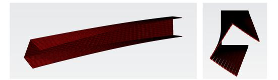
**Figure 3.** Deformation of the beam element under shear force with the AEM model (longitudinal discretisation equal to 180 and transversal discretisation of 10). It can be noted the typical coupled flexural-torsional behaviour.
