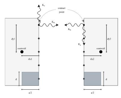
where *E* and *G* are the elastic and shear moduli, respectively; *d* is the distance between the springs; *a* is the length of the representative area; and *t* is the thickness of the element.
