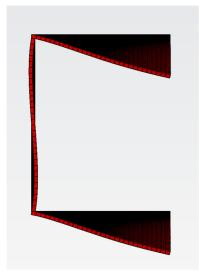
**Figure 11.** Local deformation of the flanges for Section #1, length = 100 mm, section discretisation 30 and longitudinal discretisation of 60.
