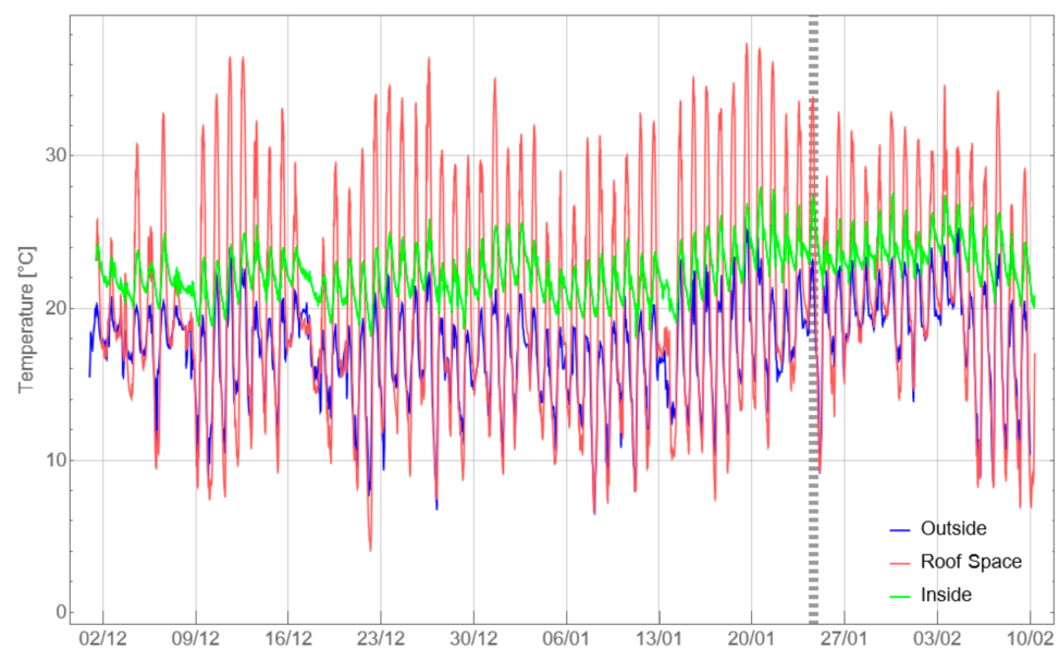
Figure 4. Temperature data from the case study dwelling during the southern hemisphere summer. The outside, roof cavity and living room data are given. The vertical dashed line represents the installation of the daytime only roof ventilator.
