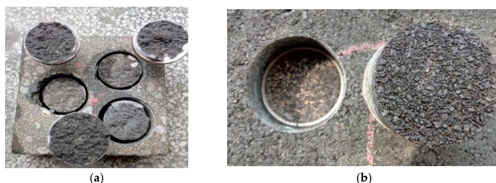
Figure 8. Drawing fracture surface of composite structure specimen: (a) Disconnection inside the mixture (b) Disconnection at the interface between the adhesive layer and the mixture.
