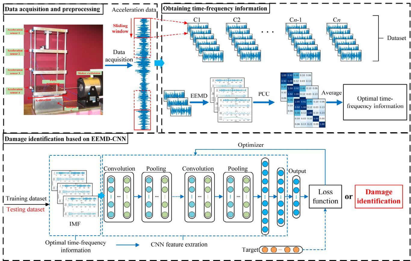
**Figure 1.** A hybrid deep learning framework for damage identification based on EEMD-PCC-CNN.
