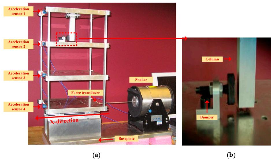
**Figure 3.** Test structure setup. (a) Three-story building structure; (b) An adjustable bumper.
