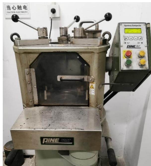
**Figure 3.** Gyrotory compactor.
