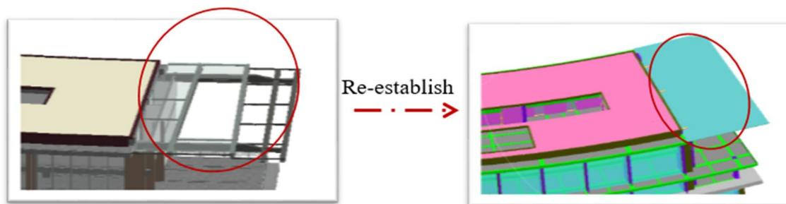
**Figure 11.** Example of a missing canopy and the need for solving the missing element.
