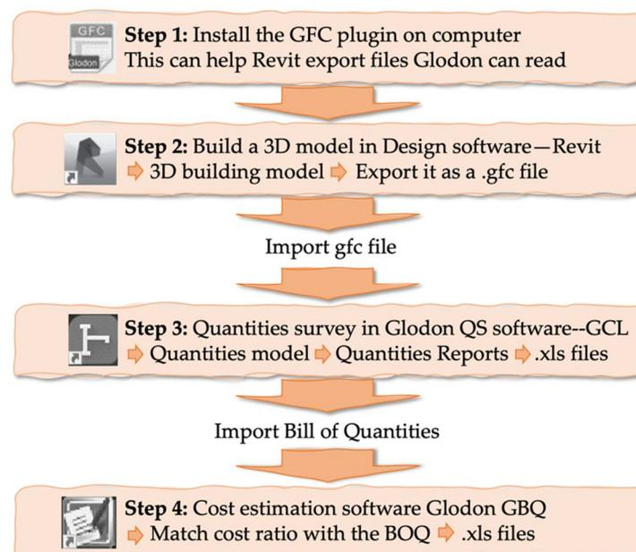
**Figure 10.** A technical workflow showing the cost estimation process using selected tools.
