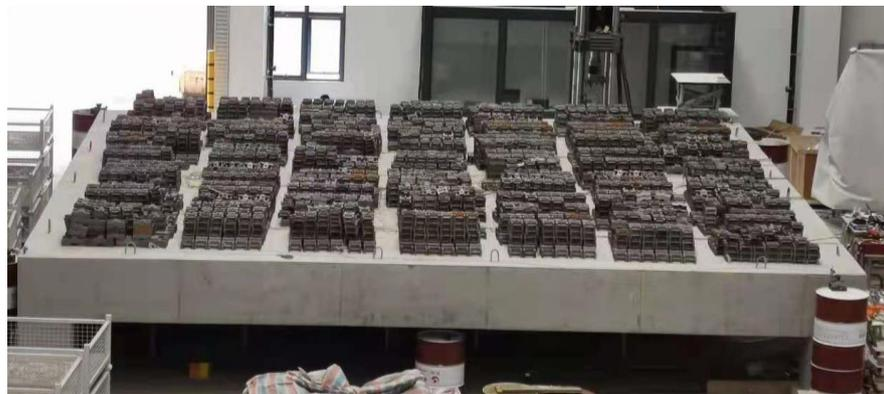
**Figure 9.** Area load exerted on the floor system.
