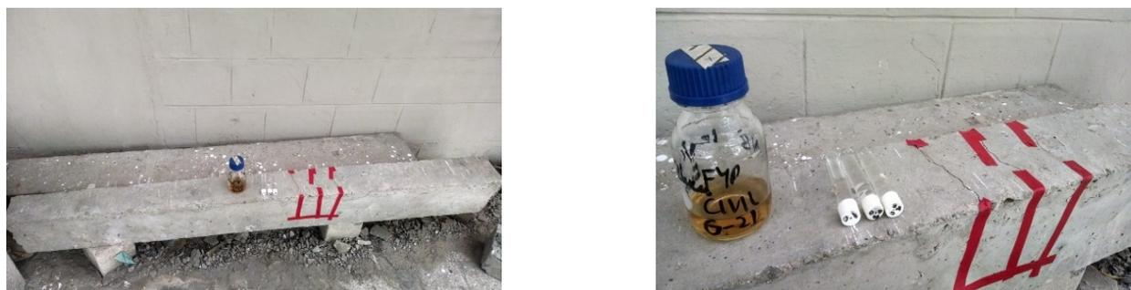
**Figure 5.** Crack-healing solution application on Beam “TCHS-1”.
