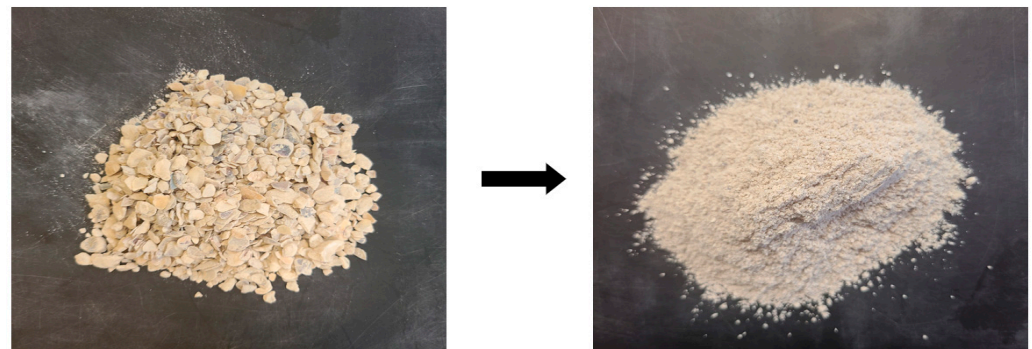
Figure 1. Process of manufacturing oyster shell powder.
