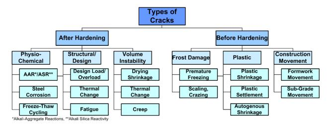
Figure 3. Common causes for cracking in concrete structures (according to [119]).
