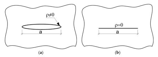
Figure 1. Diagrams of material defects in concrete: (a) crack, (b) gap [66-68].
