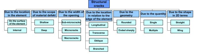
Figure 4. Breakdown of structural cracks in concrete.
