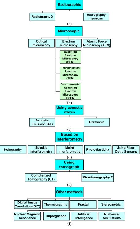
Figure 10. The most important methods for the detection and analysis of microcracks and cracks in cement concretes: (a) [185–193], (b) [173,194–204], (c) [204–213], (d) [177,214–217], (e) [179–182] and (f) [218–225].
