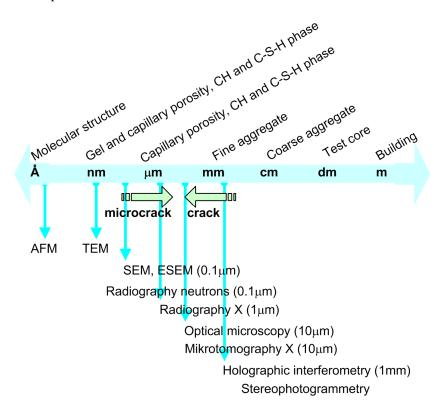
**Figure 11.** Methods for the detection of microcracks and cracks assigned to different scales of observation (according to [241]).
