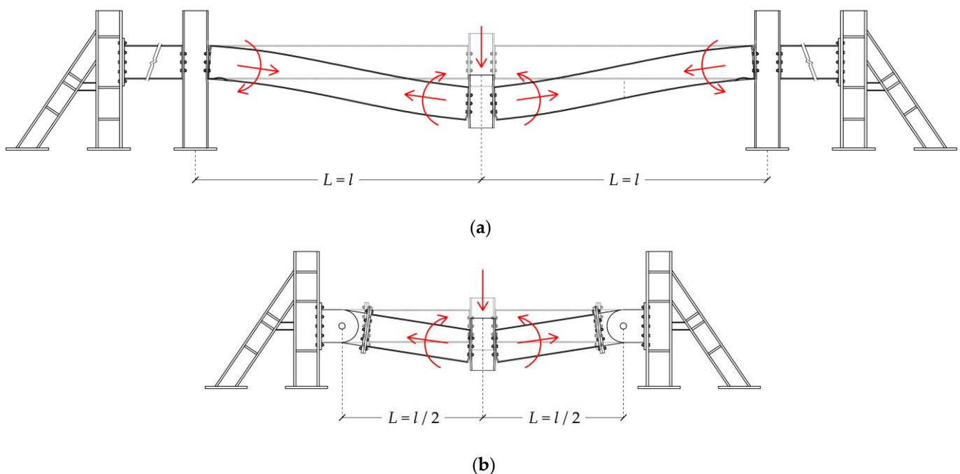
**Figure 5.** Common configurations of test specimens (where  $l$  is the span of the beam) [65]: (a) Detailed; (b) Simplified.
