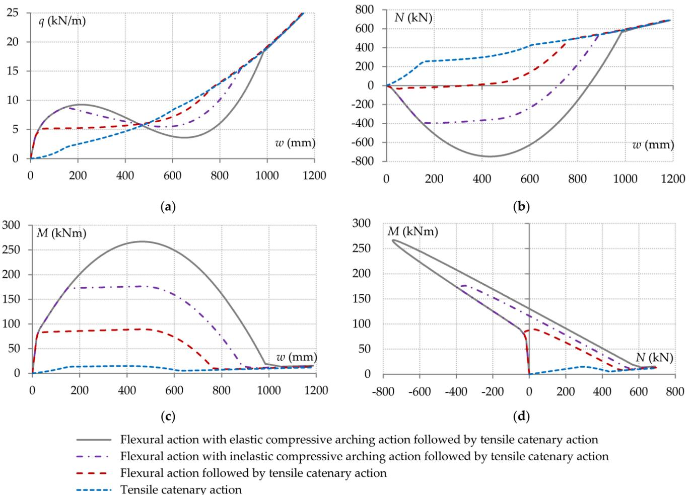
**Figure 4.** Comparison between responses governed by different collapse resistance mechanisms [57]: (a) Load–deflection curves; (b) Beam axial forces vs. beam deflections; (c) Connection bending moments vs. beam deflections; (d) Connection bending moments vs. beam axial forces.
