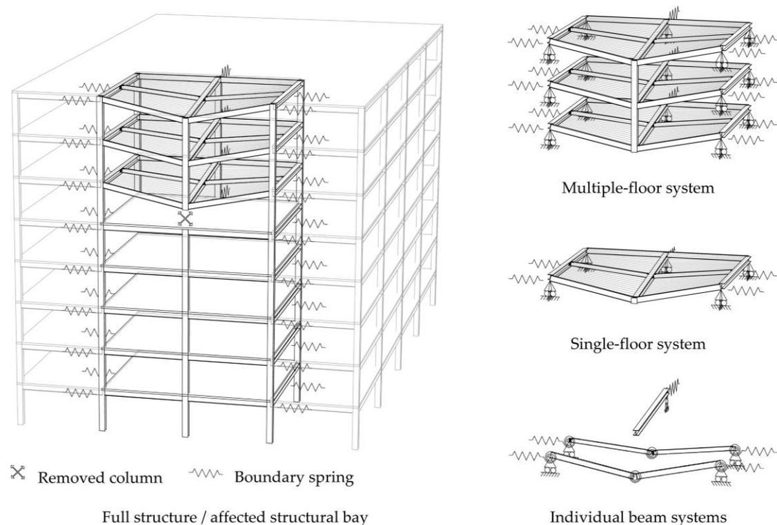
**Figure 1.** Levels of structural idealization for progressive collapse assessment [25].
