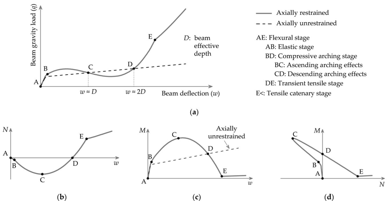
**Figure 3.** Structural response following column removal involving elastic compressive arching action [62]: (a) Beam load–deflection; (b) Beam axial force; (c) Connection bending moment; (d) Connection moment–axial force interaction.
