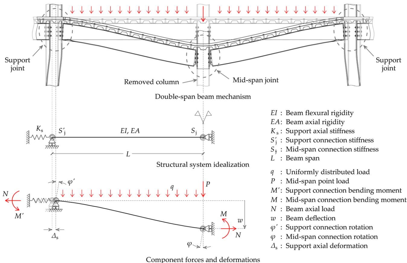
Figure 2. Representation of the double-span beam mechanism [56].
