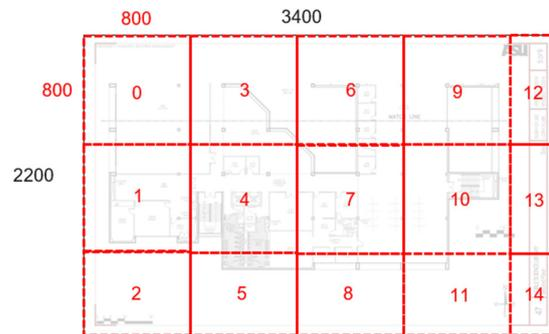
**Figure 7.** 800 × 800 pixels sliding windows sequence cropping for 3400 × 2200 pixels floor plan. (The numbers 1 to 14 indicate the sequence of crops).
