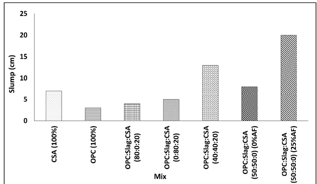
Figure 5. Measured slumps immediately after mixing the concretes.
