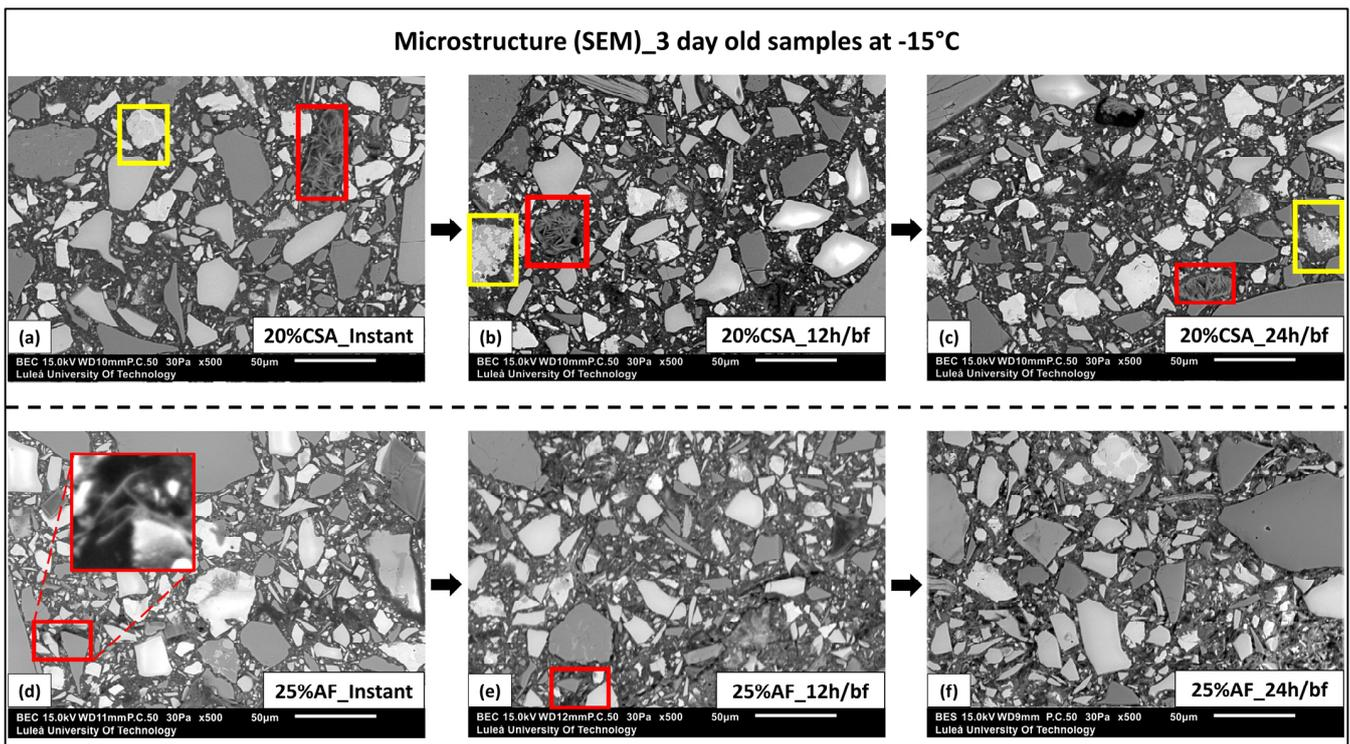
**Figure 14.** SEM images of the 3-day-old concrete samples at distinct time intervals: (a–c) OPC: GGBFS:CSA—40:40:20; (d–f) OPC:GGBFS:CSA—50:50:0 (25 wt.% of AF). (Note: Red color boxes indicate the areas with the detected ettringite crystals, and yellow boxes indicate the unhydrated CSA cement).
