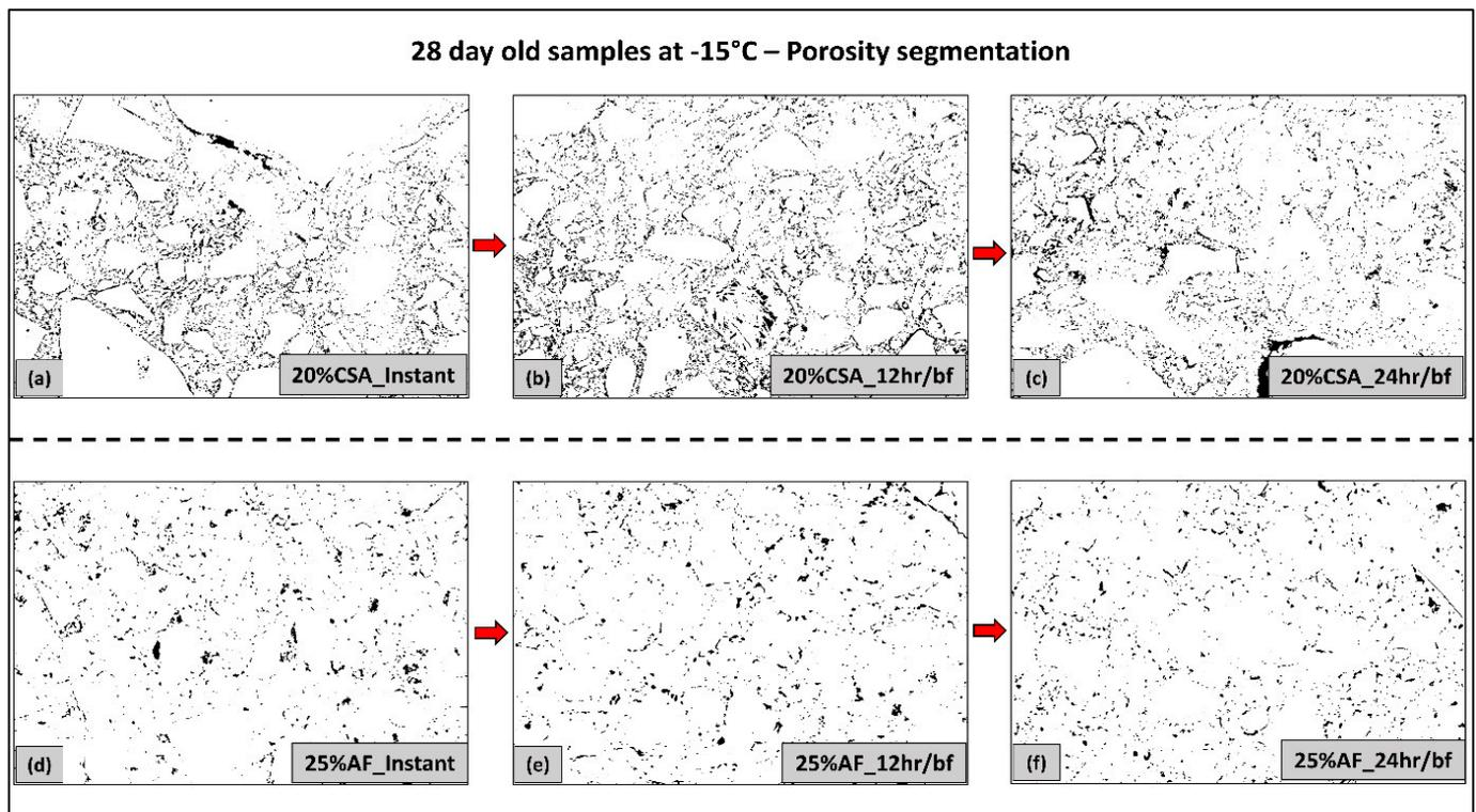
**Figure 17.** Pore segmentations on the 28-day-old concrete samples at distinct time intervals: (a–c) OPC:GGBFS:CSA—40:40:20; (d–f) OPC:GGBFS:CSA—50:50:0 (25 wt.% of AF). (**Note:** Black color indicates the pores).
