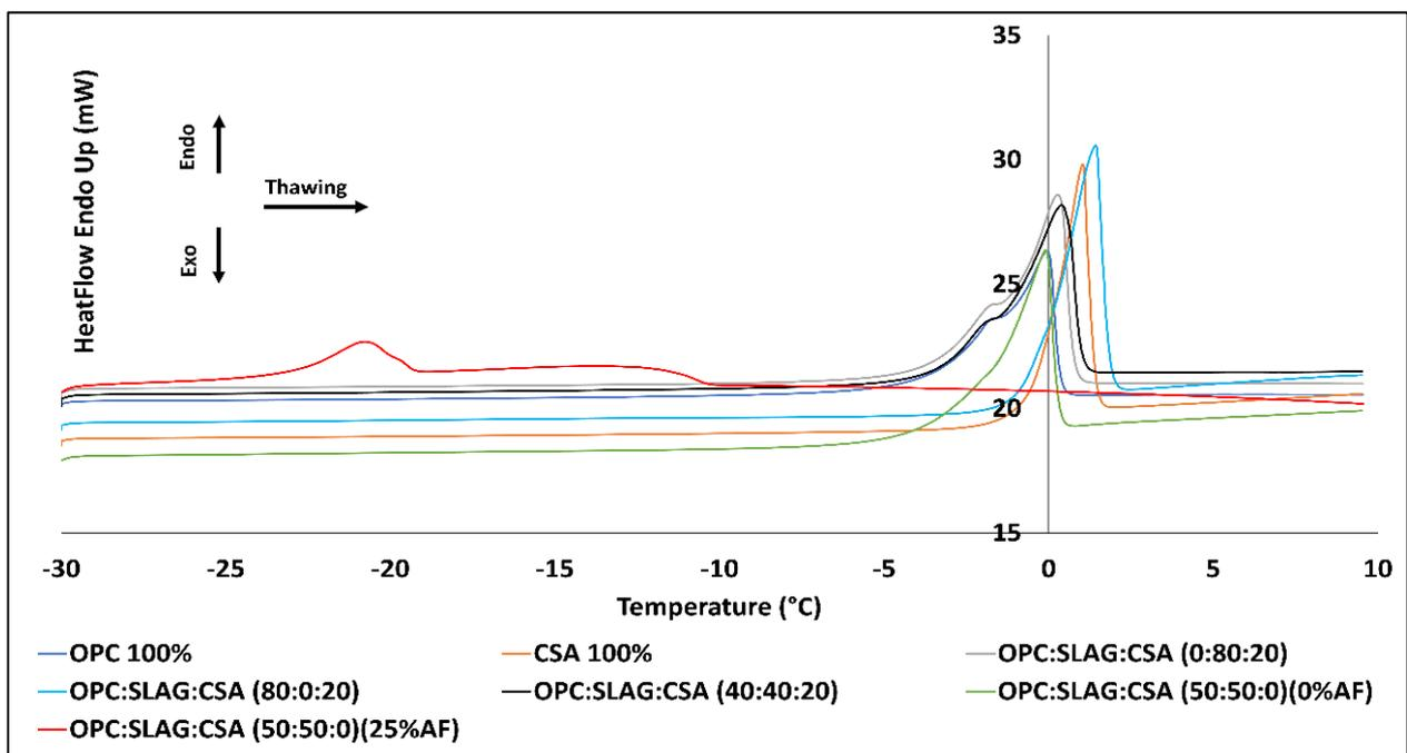
Figure 8. Endothermic heat flow of the pure OPC, CSA, and blended OPC:GGBFS:CSA pastes at a thawing rate of  $1^{\circ}/\text{min}$  using DSC.
