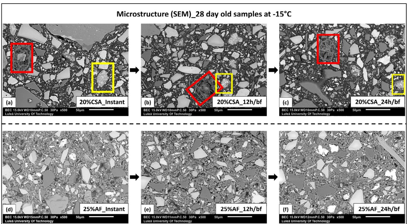
**Figure 15.** SEM images of the 28-day-old concrete samples at distinct time intervals: (a–c) OPC: GGBFS:CSA—40:40:20; (d–f) OPC:GGBFS:CSA—50:50:0 (25 wt.% of AF). (Note: Red color boxes indicate the areas with the detected ettringite crystals, and yellow boxes indicate the unhydrated CSA cement).
