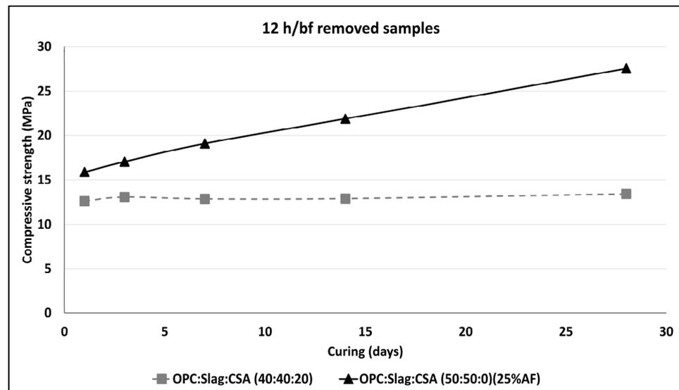
Figure 10. Strength development of the “12 h/bf” removed concrete samples cured at  $-15\text{ }^{\circ}\text{C}$ .
