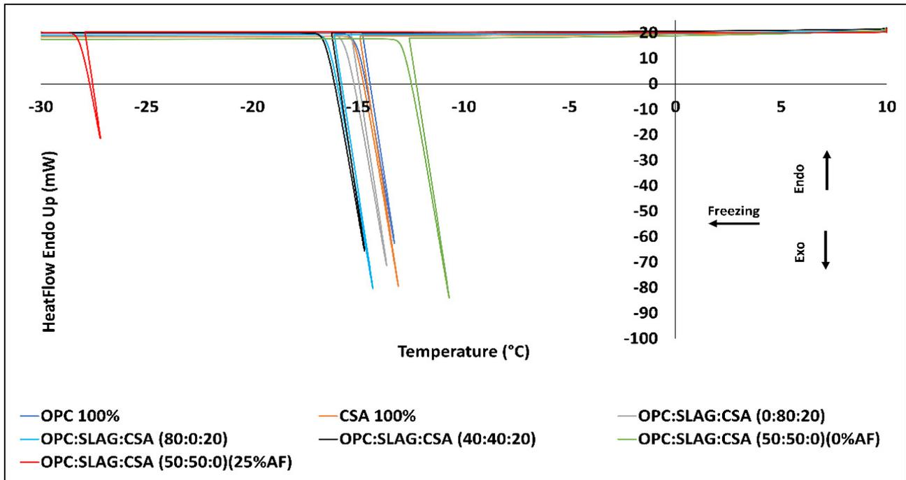
Figure 7. Exothermic heat flow of the pure OPC, CSA, and blended OPC:GGBFS:CSA pastes at a freezing rate of  $1^{\circ}/\text{min}$  using DSC.
