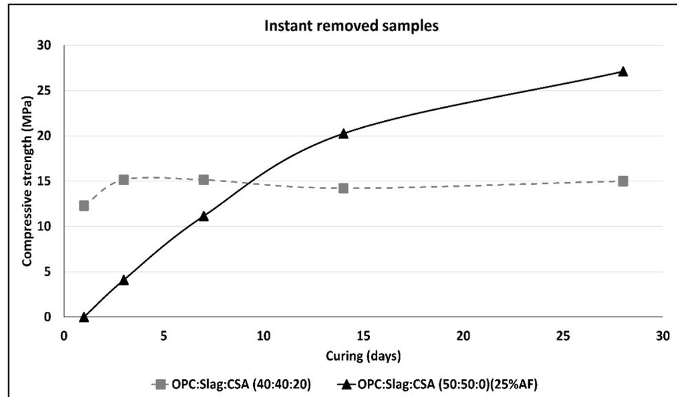
Figure 9. Strength development of the “Instant” removed concrete samples cured at  $-15\text{ }^{\circ}\text{C}$ .
