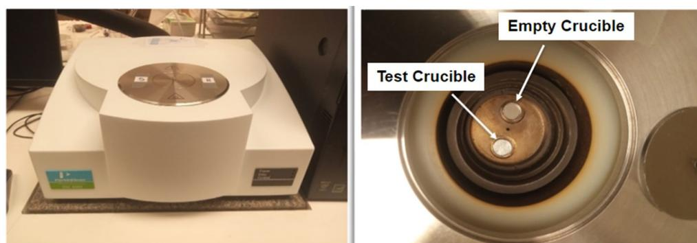
Figure 2. Differential scanning calorimetry (DSC)—Q100 TA.
