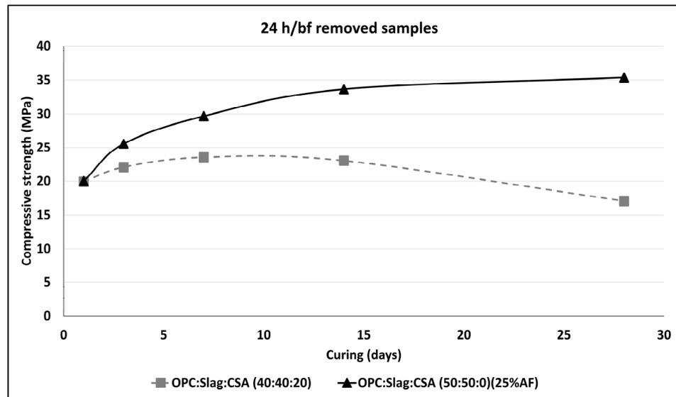
Figure 11. Strength development of the “24 h/bf” removed concrete samples cured at  $-15^{\circ}\text{C}$ .
