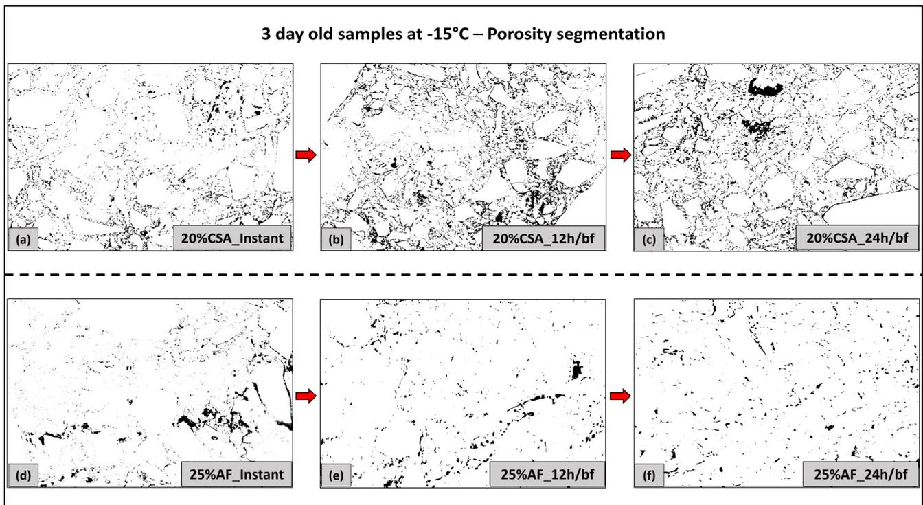
**Figure 16.** Pore segmentations on the 3-day-old concrete samples at distinct time intervals: (a–c) OPC: GGBFS:CSA—40:40:20; (d–f) OPC:GGBFS:CSA—50:50:0 (25 wt.% of AF). (**Note:** Black color indicates the pores).
