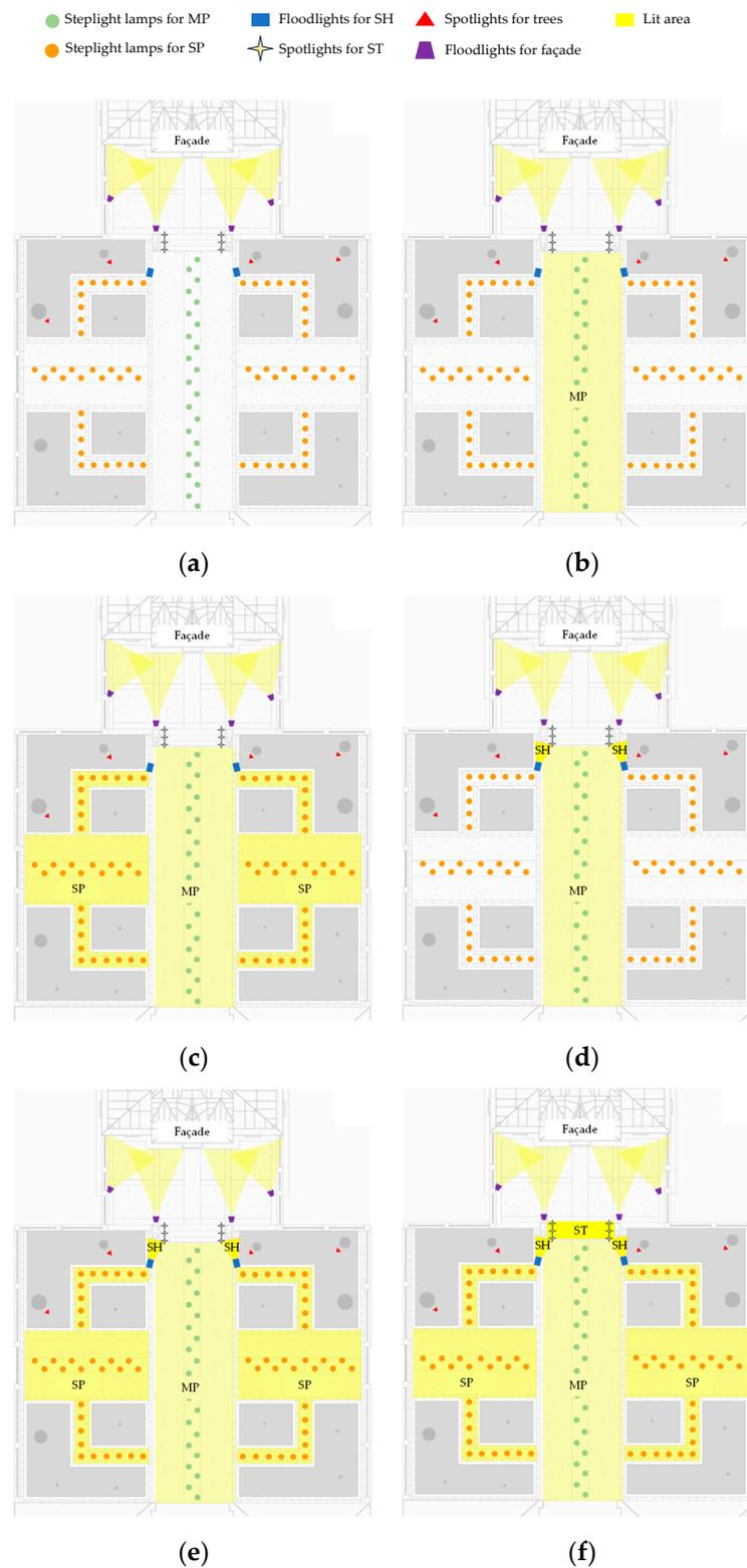
**Figure 5.** Layout of the luminaires' position and the illuminated areas of the garden upon varying the scenic elements: (a) Scenario 1; (b) Scenario 2; (c) Scenario 3; (d) Scenario 4; (e) Scenario 5; (f) Scenario 6.
