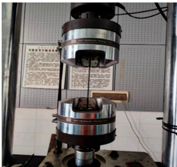
**Figure 3.** Loading equipment of the SMA rod.
