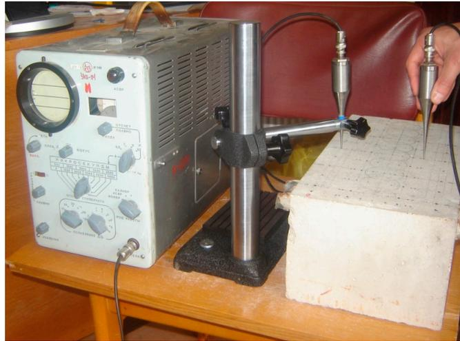
**Figure 2.** The oscillograph “UKB-1M” device applied for the measurement of a reinforced concrete specimen [1].
