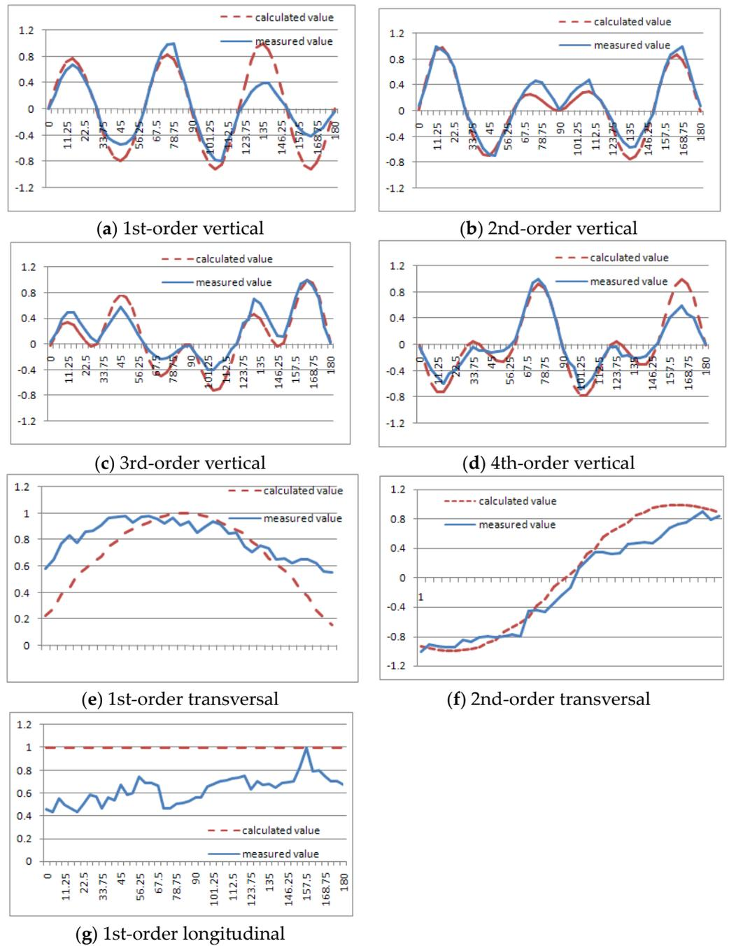
Figure 6. Comparison of modal vibration shape between the testing and calculation.
