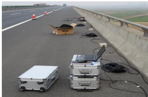
**Figure 2.** Sensor arrangement for environment vibration.
