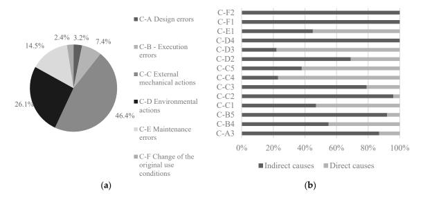
**Figure 6.** Probable causes of anomalies: (**a**) Relative frequency of each group of causes; and (**b**) direct vs. indirect causes.
