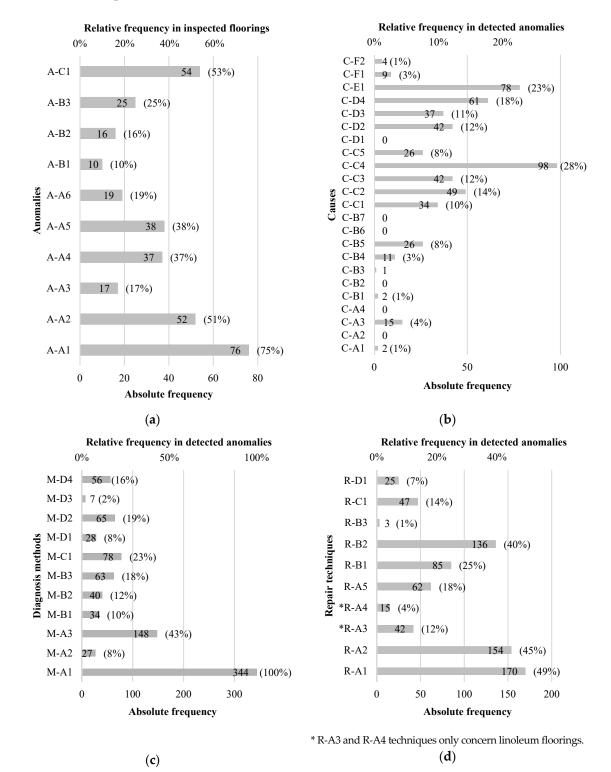
**Figure 2.** Absolute frequency (and relative frequency) of: (**a**) Detected anomalies; (**b**) probable causes; (**c**) adequate diagnosis methods; (**d**) recommended repair techniques.
