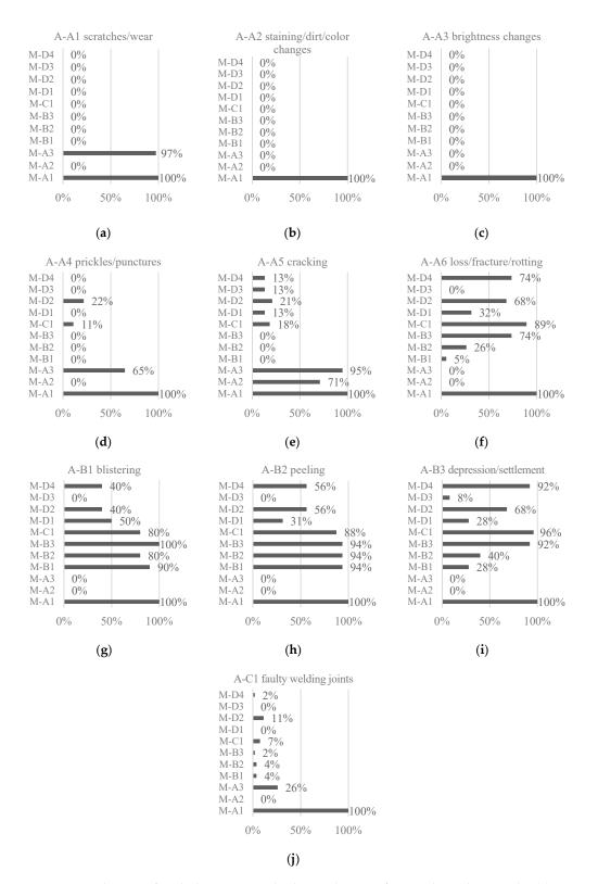
**Figure 8.** Contribution of each diagnosis method to each type of anomaly in the sample: (**a**) A-A1 scratches/wear; (**b**) A-A2 staining/dirt/color changes; (**c**) A-A3 brightness changes; (**d**) A-A4 prickles/ punctures; (**e**) A-A5 cracking; (**f**) A-A6 loss/fracture/rotting; (**g**) A-B1 blistering; (**h**) A-B2 peeling; (**i**) A-B3 depression/settlement; (**j**) A-C1 faulty welding joints.
