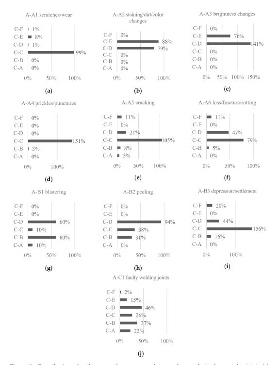
**Figure 7.** Contribution of each group of causes to each type of anomaly in the sample: (**a**) A-A1 scratches/wear; (**b**) A-A2 staining/dirt/color changes; (**c**) A-A3 brightness changes; (**d**) A-A4 prickles/ punctures; (**e**) A-A5 cracking; (**f**) A-A6 loss/fracture/rotting; (**g**) A-B1 blistering; (**h**) A-B2 peeling; (**i**) A-B3 depression/settlement; (**j**) A-C1 faulty welding joints.
