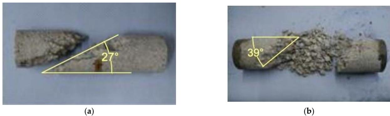
**Figure 7.** Typical fracture pattern; (a) test series P0 and PE; (b) test series A10 and A20.
