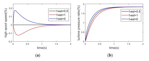
Figure 10. FTC result in different fault reconstruction (FC) situations. (a) controlled variables (b) control variables.
