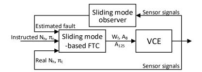
Figure 2. Structure of the actuator fault tolerant control design.
