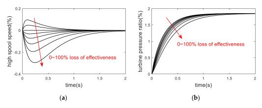
**Figure 5.** Fault tolerant control (FTC) result of sliding mode control (SMC) design-controlled variables. (a)  $n_{t}$  (b)  $\pi_{t}$ .
