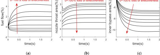
**Figure 9.** FTC result of ASMC design-control variables. (a)  $W_f$  (b)  $A_8$  (c)  $A_{125}$ .
