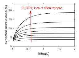
**Figure 7.** Expected nozzle throat area of *A*<sup>8</sup> in SMC design.
