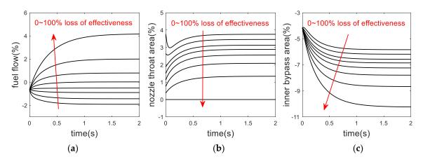
**Figure 6.** FTC result of SMC design-control variables. (a)  $W_f$  (b)  $A_8$  (c)  $A_{125}$ .
