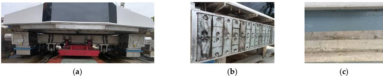
**Figure 1.** An HTS maglev test vehicle equipped with PMECBs: (a) the test vehicle; (b) the PMECB composed of Halbach permanent magnet array fixed on both sides of the vehicle; (c) the metal induction plates.
