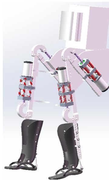
**Figure 1.** 3D model of lower limb exoskeleton rehabilitation robot.
