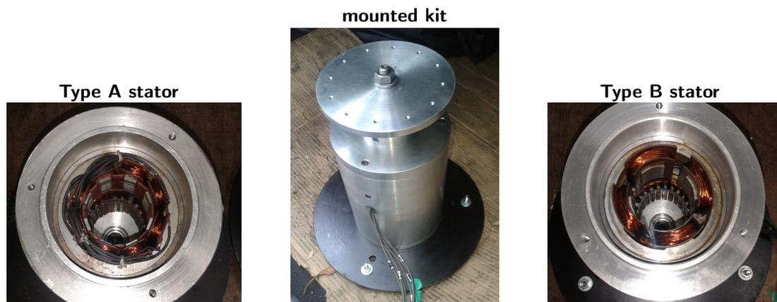
**Figure 9.** Top view of Prototypes A, on the left, and B, on the right; notice the eight “poles” in Type A and only four “poles” in Type B. A mounted kit is shown in the center, with a vertical rotor inserted in one of the carcasses. The perforated disk built in the upper position is used for mass unbalance tests.
