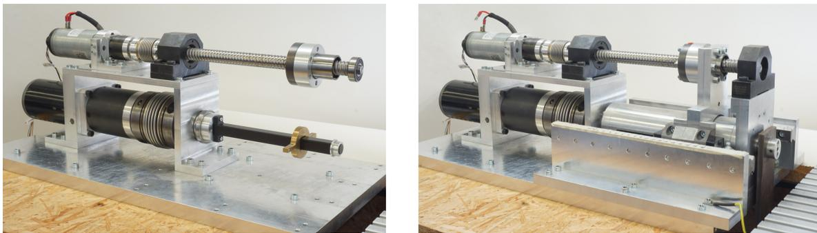
**Figure 8.** Variable torsion stiffness actuator; partially disassembled (left) and assembled (right).
