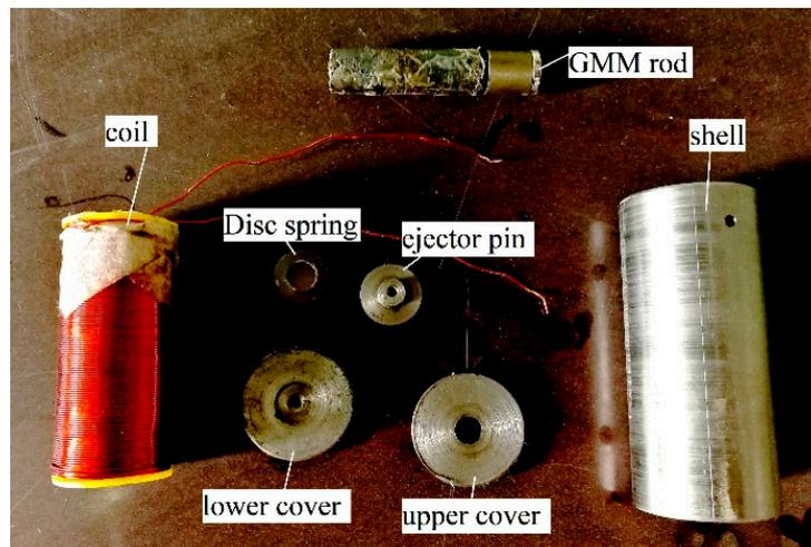
Figure 10. Prototype of SGMA.
