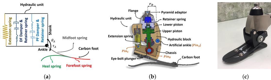
**Figure 1.** Spring and dampers structure in a simple mechanical model (a), CAD representation (b), final fabricated model (c) of the H2AP. The hydraulic block included DF and PF dampers. DF and PF stand for dorsiflexion and plantar flexion, respectively. The carbon foot comprises three interlocked springs. Ankle torque and ankle angle are shown by  $\tau_A$  and  $\theta_A$ , accordingly.
