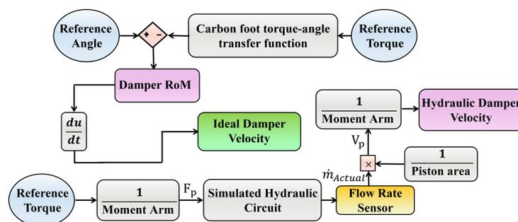
**Figure 6.** The flowchart algorithm for determining the rotary flow control valves' diameter range for operating in the simulated hydraulic circuit and optimal diameter to adjust optimal flow rate.
