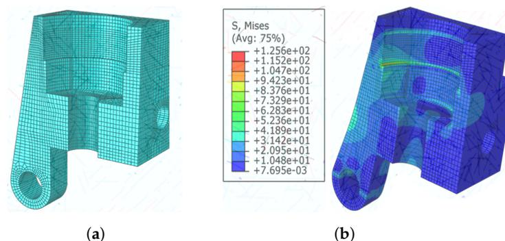
**Figure 8.** A simplified model associated with a suitable mesh size (a) and stress analysis (b) of the hydraulic block. The stress analysis was performed using ABAQUS.
