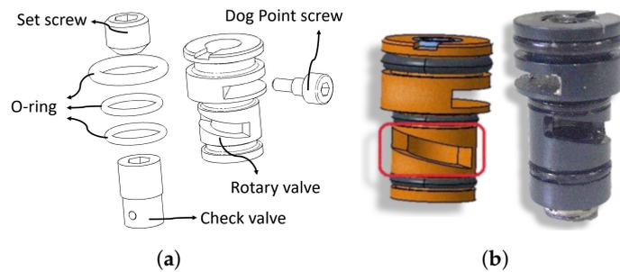
**Figure 3.** Exploded view (a) and final CAD and fabricated model (b) of the proposed rotary flow control valve embedded in the H2AP hydraulic damper.
