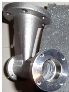
**Figure 8.** Dust accumulated inside the cyclone, behind the skimmer region. The dust particles deposited by the path of the swirling collection liquid.
