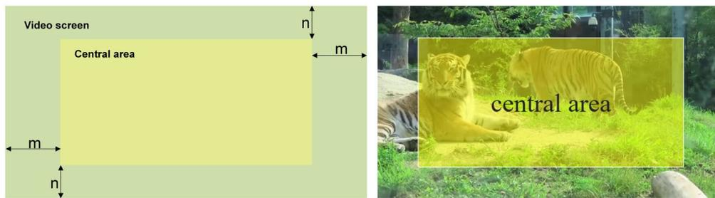
**Figure 6.** Schematic diagram of the division of the central area. The diagram on the left is an abstract representation, where we defined the central area as a fixed-scale area at the boundary of the video screen. The real situation is shown in the diagram on the right.
