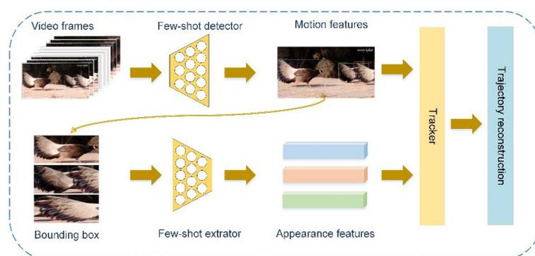
**Figure 1.** We aimed to obtain a few-shot multiobject-tracking model based on few-shot learning. In this framework, we used a few-shot object detector as the detector and a classification network trained based on the few-shot method as the feature extractor. In addition, we also designed a trajectory-reconstruction module to optimize the tracking result.
