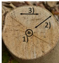
**Figure 1.** Anisotropy axes of wood: (1) in the fiber direction; (2) in the direction across the fiber, radial to the annual rings; (3) in the direction across the fiber, tangential to the annual rings.
