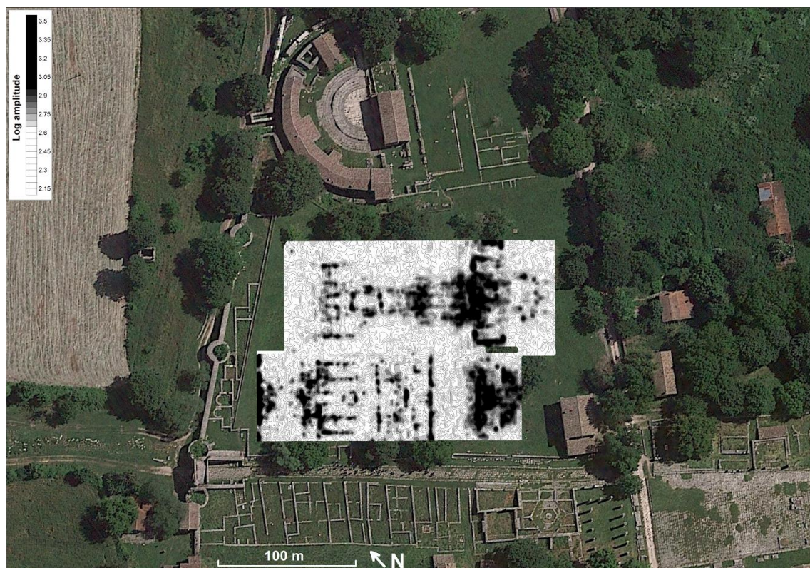
Figure 8. Time slice relative to 14–18 ns overlapped to a Google Earth™ satellite image.
