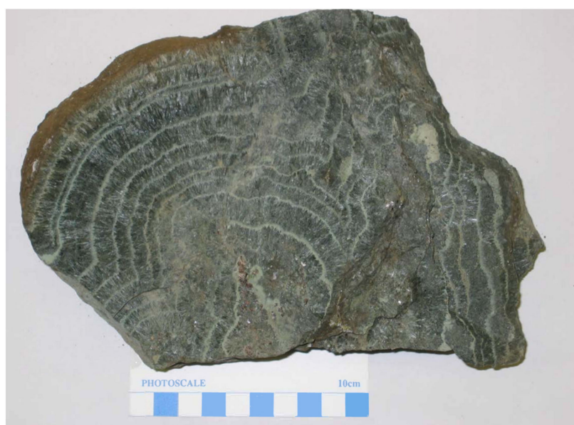
Figure 2. A typical Mokuji ore (hedenbergite with sphalerite and galena) from Maebira, –315 mL, 5 Otsu-3 of the Tochibora deposit.
