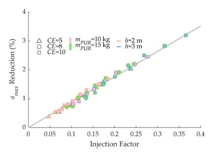
**Figure 14.** Reduction of surficial accelerations in relation to the injection factor, representative of the number of injections, mass of injected polyurethane, depth of injected soil, as well as the soil stiffness.
