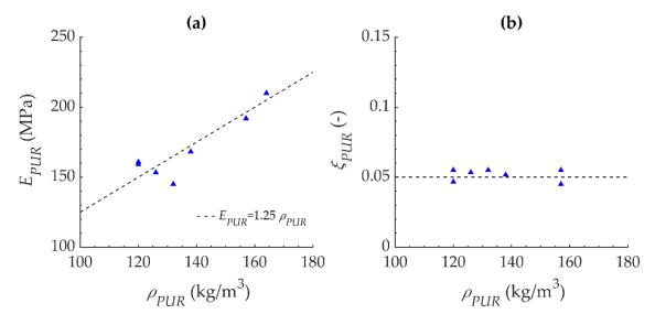
**Figure 9.** Parameters obtained from the elaboration of impact test results. Variation with polyurethane density of (a) the elastic modulus and (b) the damping coefficient.
