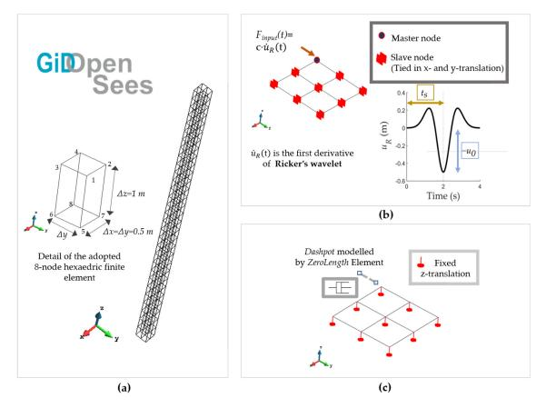
**Figure 4.** FE numerical modelling: (a) 3D model and finite element adopted, (b) input application at an end node of the base, with master-slave node for uniform excitation introduction, and (c) modelling of a viscous-elastic bedrock.
