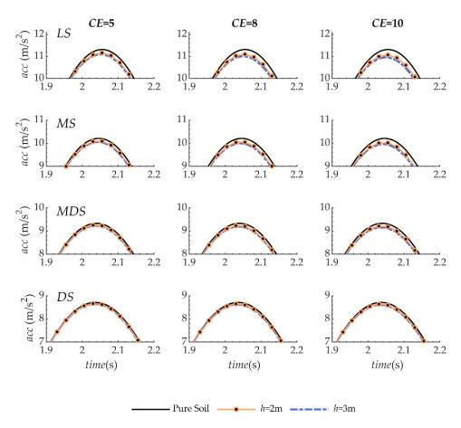
**Figure 10.** Time-history accelerations recorded on numerical models of pure cohesionless soil at different relative densities and on "modified" cohesionless soil: evidence of the effects of the thickness of the modified layer ( $m_{PUR} = 15$  kg injected per level).
