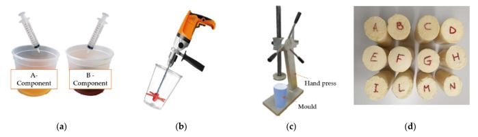
**Figure 2.** Sample preparation: (a) Sampling of the two components with syringes (Volume ratio 1:1), (b) injection of both components into a plastic cup being mixed through a propeller-equipped drill, (c) outpour of the mixed foam inside a mould, closed by a hand press, and (d) specimens for tests.
