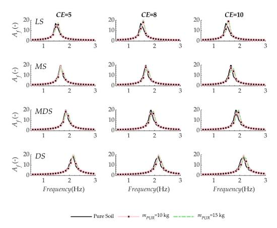
**Figure 13.** Amplification functions for h = 3 m and  $m_{PUR} = 10$  and 15 kg.
