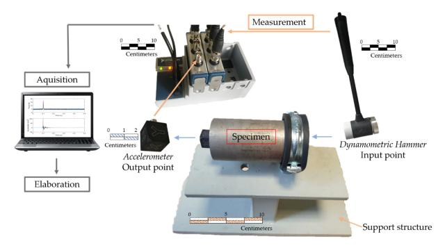
Figure 3. Scheme of the impact test performed, with details of the instruments used.
