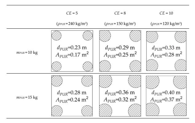
**Figure 5.** Summary of the injection cases analysed. The polyurethane diameter and area are shown, corresponding to each considered combination injected mass per level,  $m_{PUR}$ —expansion coefficients CE.
