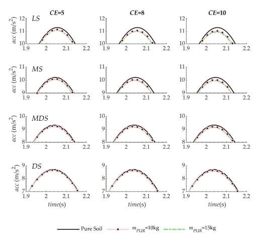
**Figure 11.** Time-history accelerations recorded on numerical models of pure cohesionless soil at different relative densities and on "modified" cohesionless soil: evidence of the effects of the mass injected per level (h = 3 m).
