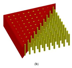
**Figure 1.** Polyurethane injection scheme underneath foundation slabs: (a) Application example realised by Bequadro S.r.l., and (b) schematisation of polyurethane injections as cylinders (green) in the soil matrix (red).
