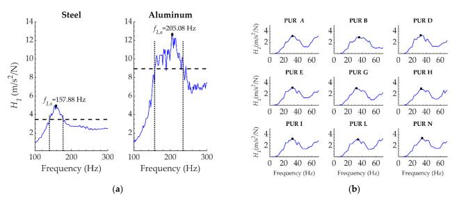
**Figure 8.** Frequency response functions,  $H_1$ , for (a) steel and aluminium specimens and (b) polyurethane specimens at different densities. In both figures, the marker shows the fundamental frequencies; in Figure (a), the application of the half-power bandwidth method for the damping evaluation is also illustrated.
