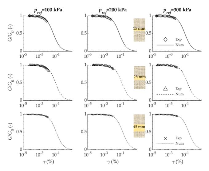
**Figure 6.** Numerical (Num) vs. experimental (Exp) comparison of the shear modulus decay for composite sand-polyurethane samples at three thicknesses (15, 25 and 45 mm) and for three confining pressures.
