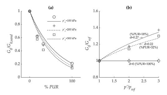
**Figure 7.** Homogenisation procedure of the small-strain parameters for the composite specimens. (a) Experimental (points) vs. analytical (lines)  $G_0/G_{0,sand}$  varying with the polyurethane volumetric percentage. (b) Calibration of d exponent for shear modulus variation with the isotropic stress.
