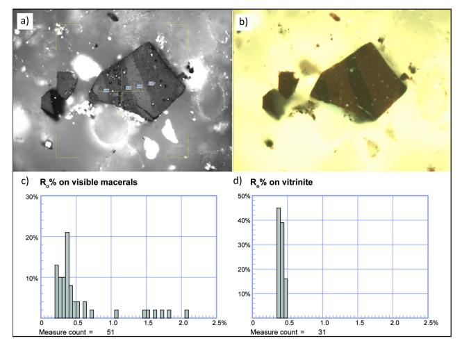
**Figure 4.** Examples of reflected light images of the analysed macerals: (**a**) Lithotype composed by vitrinite (light portion of the fragment) and liptinite (dark part); (**b**) same fragment of figure A observed under fluorescent light. It can be noted the weak brownish fluorescence of liptinite. Example of a Random Reflectance histogram showing: (**c**) reflectance of all visible macerals and (**d**) only vitrinite in the same sample.
