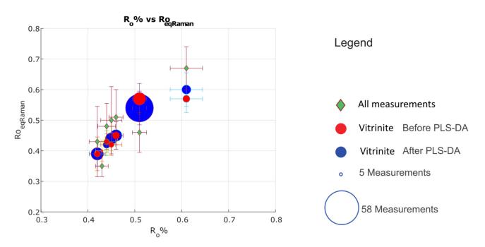
**Figure 8.** The diagram shows the correlation between the microscopic determination of vitrinite reflectance ( $R_0$ %) and the reflectance equivalent of vitrinite ( $R_{oeq}$ %) macerals calculated by means of Raman parameters, according to [38], for values obtained before (red circles) and after (blue circles) PLS-DA analysis. The size of the circles depends on the number of measurements for each sample. Green diamonds show  $R_{oeq}$ % values calculated on all macerals composition.
