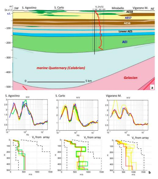
**Figure 18.** (a) Geological cross-section from Sant'Agostino to Vigarano Mainarda [19] and Vs profile from Mirabello down-hole [36], (b) H/V spectral ratios and Vs profiles from ambient vibration measurements (array) [19].
