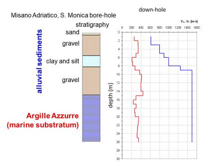
**Figure 7.** Example of stratigraphic log and Vs-Vp profiles (down-hole) in the foothills area (Santa Monica site, Misano Adriatico Municipality, Rimini Province).
