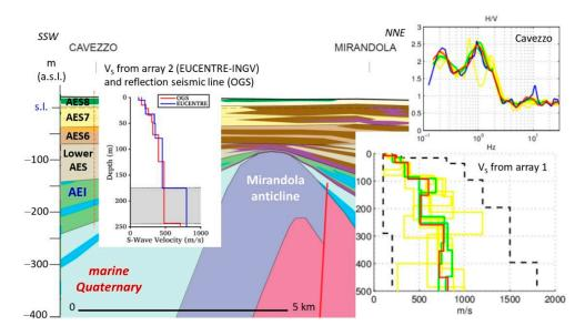
**Figure 19.** Geological cross-section from Cavezzo to Mirandola, H/V spectral ratio and Vs profile from ambient vibration measurement (array) in the Cavezzo urban area [19] and Vs profiles from Cavezzo seismic microzonation [26].
