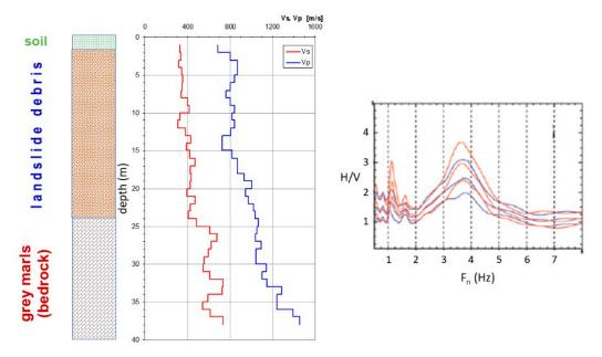
**Figure 1.** Comparison between stratigraphic log, Vs profiles from down-hole and ambient noise in an Apennines site characterised by debris cover (landslide) on marly geological substratum (modified from [10]).
