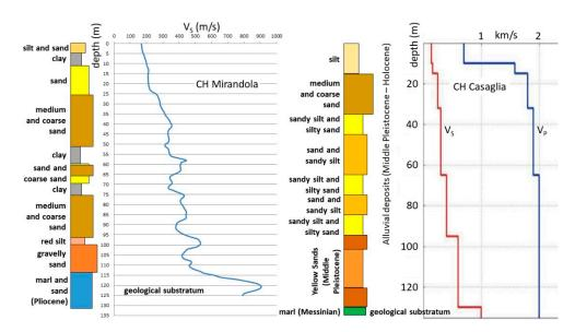
Figure 15. Stratigraphic logs and Vs profiles in Mirandola and Casaglia [19,22].
