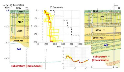
**Figure 20.** Geological cross-section along the coast from Cesenatico to Viserba (from Geological Map of Italy, sheet no. 256 "Rimini"), H/V spectral ratio and Vs profile from ambient vibration measurement (array) in the Cesenatico urban area [38].
