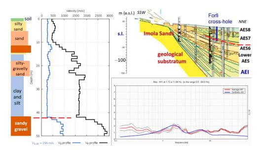
**Figure 8.** Stratigraphic log, Vs-Vp profiles (cross-hole, from http://itaca.mi.ingv.it/ItacaNet\_30/#/station/IT/FOR, with modifications, accessed on 1 July 2021) and ambient noise measurement (from seismic microzonation, Forlì Municipality) in the Forlì station of the National Accelerometric Network; geological cross-section from CARG 1:50,000, sheet n. 240 "Ravenna".
