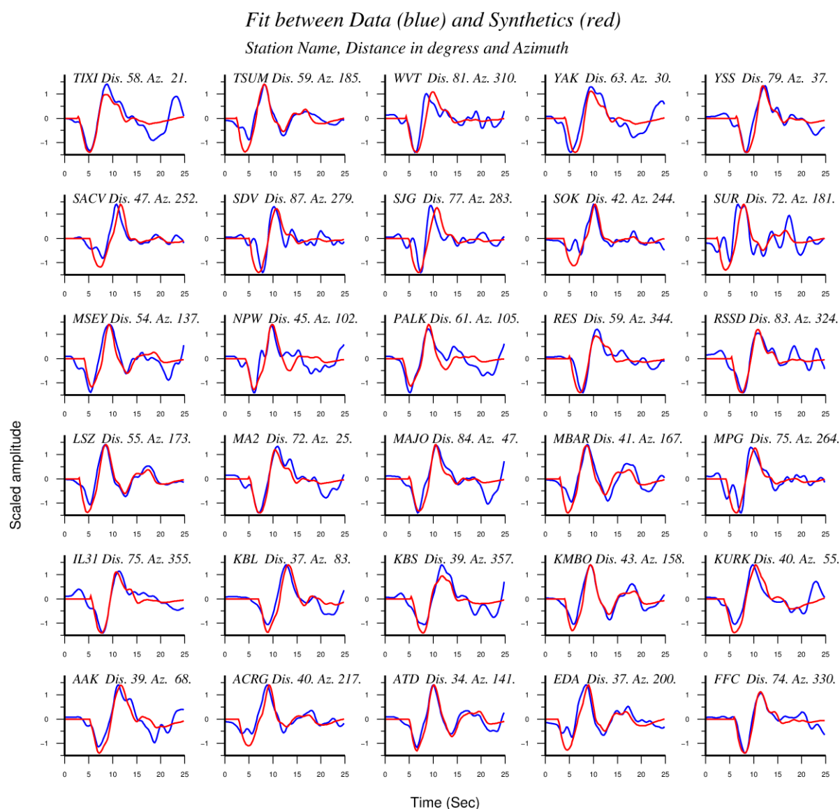
Figure 5. Scaled fit between real waveforms (blue lines) and synthetics (red lines) for the 30 stations; station name (e.g., TIXI), station epicentral distance in degrees (Dis.) and azimuth (Az.) are also shown.
