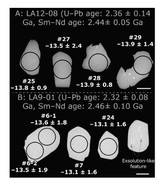
**Figure 2.** Representative BSE images of apatite crystals from the amphibolite facies grey gneiss LA12-08 (panel **A**) and metatexite LA9-01 (panel **B**). Scale bars represent 100  $\mu$ m. Spot size: 130  $\mu$ m. Labels represent analysis number (#) and  $\epsilon^{143}$ Nd<sub>initial</sub> deviation  $\pm$  uncertainty at 95% confidence level calculated at the Sm–Nd isochron apparent age for each apatite population.
