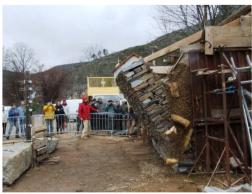
**Figure 8.** Picture of the "C3s" DSRWs tested by A.S. Colas: initial and collapse configurations are shown [43].
