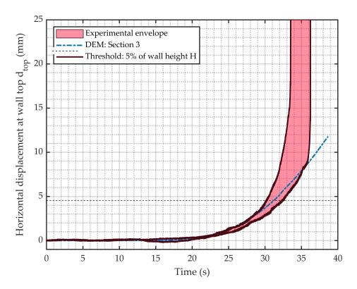
**Figure 7.** Comparison of experimental and numerical responses for a wall with a slenderness of H/B = 2.3 subjected to a dynamic input of 30 Hz.
