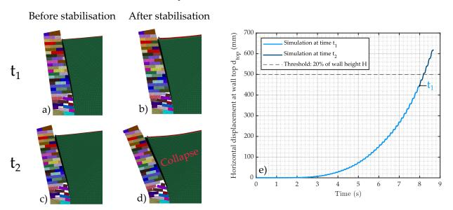
**Figure 13.** Definition of the threshold indicating the DSRW's collapse using the input signal  $S_2(t)$ . (a) DSRW1 at simulation time  $t_1$ ; (b) DSRW1's stabilisation under vertical gravity only, starting from simulation time  $t_1$ ; (c) DSRW1 at simulation time  $t_2$ ; (d) DSRW1's stabilisation under vertical gravity only, starting from simulation time  $t_2$ ; (e) comparison of the obtained displacement up to simulation times  $t_1$  and  $t_2$ .
