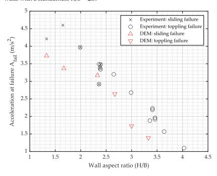
**Figure 6.** Comparison of the acceleration at failure ( $A_{fail}$ ) between the numerical simulations and experimental tests for different wall slenderness (H/B).
