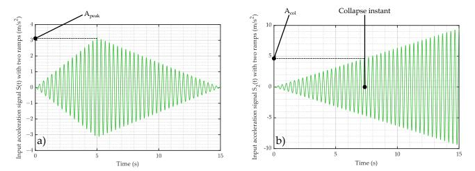
**Figure 12.** Example of the harmonic input signals S(t) used in the numerical simulation of full-scale DSRWs with a frequency of f = 3Hz. (a)  $S_1(t)$ : signal with two ramps, idealising a seismic signal and (b)  $S_2(t)$ : signal with an infinitely increasing ramp. Note that the increasing ramps of both signals have the same slope.
