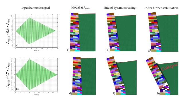
**Figure 14.** Evaluation of the ratio between  $A_{peak}$  and  $A_{col}$  for DSRW1: (a) dynamic input signal with  $A_{peak} = 0.6 \times A_{col}$ ; (b) dynamic input signal with  $A_{peak} = 0.7 \times A_{col}$ ; (c,d) models at  $A_{peak}$ ; (e,f) models at the end of the dynamic input; (g,h) computation of the post-seismic static equilibrium.
