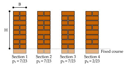
**Figure 3.** Four different cross-sections in the wall length illustrated for the walls with a slenderness H/B = 2.7. Recall that H refers to the wall height free to move throughout the shaking, disregarding the first fixed masonry course.
