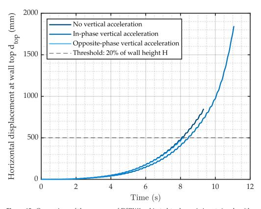
**Figure 15.** Comparison of the response of DSRW1 subjected to dynamic input signals with and without vertical acceleration.
