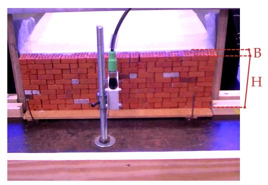
**Figure 2.** Retaining wall mock-up [33], for a wall of slenderness H/B = 3.3.
