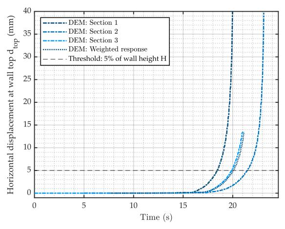
**Figure 4.** Comparison of the displacement at the top of the wall (slenderness H/B = 2.7) for the different cross-sections (Figure 3) and the global weighted response.
