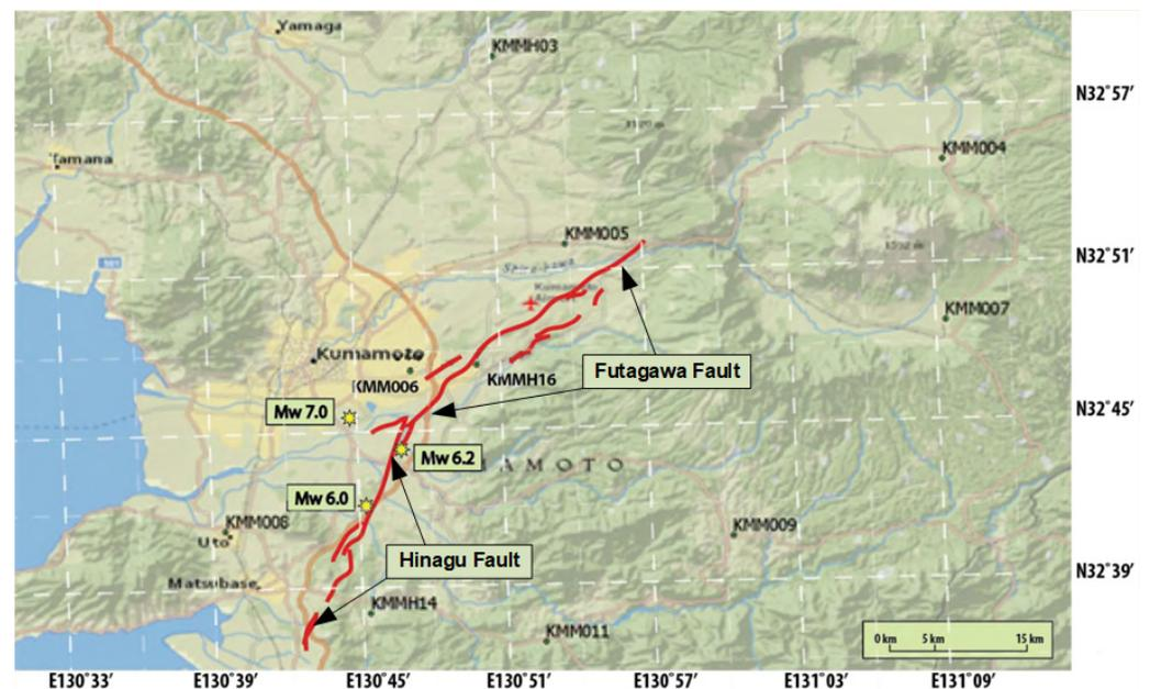
**Figure 4.** Map of the foreshock and mainshock epicenters, the Futagawa and Hinagu faults, and the ground motion recording stations listed in Table 1. Red lines represent faults, stars represent epicentral locations for earthquake events in the 2016 KES.
