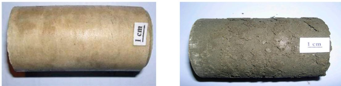
**Figure 3.** General view of frozen sand samples with pore hydrates and massive ice–hydrate texture (at  $-6$  to  $-7$  °C and  $0.1$  MPa).
