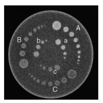
**Figure 1.** A Phantom of low contrast module. Six different regions have been depicted where low contrast objects are put (A–C and a–c). Low cylindrical objects were placed in Regions A–C to contrast the difference in the objects in Regions A/a, B/b and C/c with the backgrounds of 1%, 0.5% and 0.3%, respectively.
