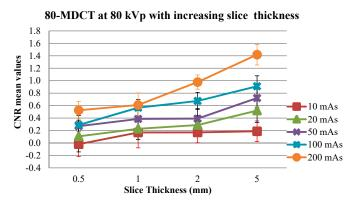
**Figure 3.** Thicker slice images resulted in higher CNR values at 80 kVp with different mAs levels for the 80-MDCT scanner. (Note the change in CNR values at 10 mAs among 1-, 2- and 5-mm slice thickness images and the change in CNR values at 50 mAs between 1- and 2-mm slice thickness images.)
