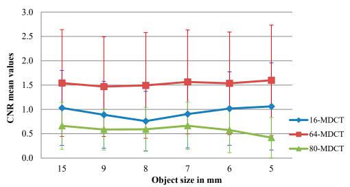
CNR of 1% contrast level objects of different size in different MDCT scanners
