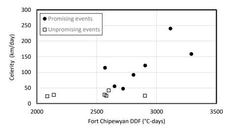
**Figure 8.** Celerities of promising and unpromising events plotted versus cumulative degree-days of frost at Fort Chipewyan.
