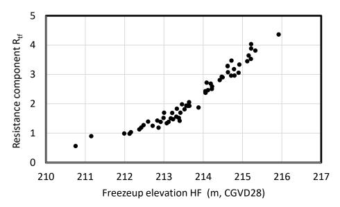
**Figure 10.** Variation of the resistance component  $R_{tf}$  with the freezeup level for the vicinity of the Peace Point hydrometric gauge, 1962 to 2020 data. For Peace Point, the highest known HF is ~215.9 m; HR is taken as 216.0 m.
