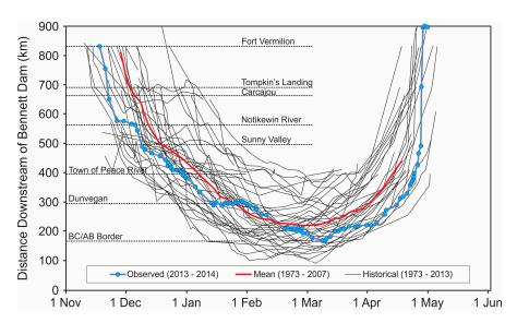
**Figure 2.** Observed locations of Peace River ice front downstream of Bennett Dam. From Alberta Environment archived material, 1973–2014, with changes. https://rivers.alberta.ca/apps/Basins/data/figures/river/abrivers/RFSPubArchive/RiverIce/pubs/2013-2014\_Peace\_River\_Ice\_Obs\_Rpr\_No46.pdf (accessed on 4 October 2023).
