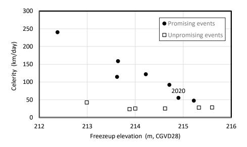
**Figure 9.** Celerities of promising and unpromising events plotted versus freezeup level at Peace Point. In 2020, the freezeup level may have been as high as 215.5 m, moving the plotted point "eastward".
