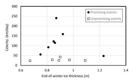
**Figure 7.** Celerities of promising and unpromising events plotted versus ice cover thickness at Peace Point.
