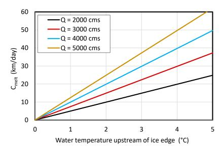
**Figure 3.** Thermal advance of the breakup front as a function of flow and upstream water temperature (Equation (1)) for a 600 m wide rectangular channel, assuming 0.8 m thick sheet ice cover.
