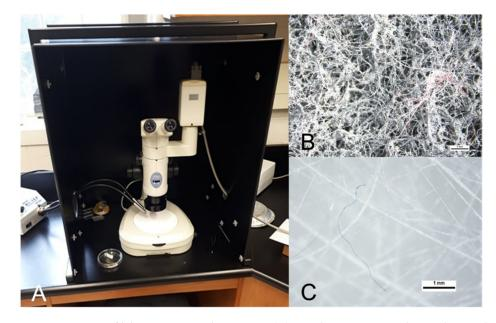
**Figure 1.** Images of laboratory control measures. (**A**) Metal microscope enclosure designed to reduce background contamination. (**B**) Microfibres entangled within a black carbon filter examined from a HEPA air purifier. (**C**) A blue fibre identified in a glass-fibre filter from an air exhaust unit.
