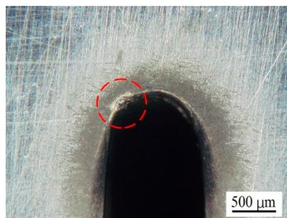
Figure 14. Surface with burns.
