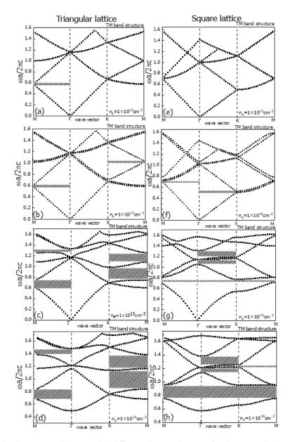
**Figure 4.** The dispersion relations under different electron densities for the triangular lattice (**a-d**) and the square lattice (**e-h**) shown in Figure 2a,b. The shadow strips indicate the positions of the band gaps. The plasma collision frequency  $v_m = 160$  GHz.
