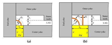
**Figure 4.** Models of permanent magnet (PM)-to-yoke magnetic flux leakage: (a) Circular-arc model for the case of  $h_m < T_s + \delta$ ; (b) circular-arc and straight-line model for the case of  $h_m > T_s + \delta$ .
