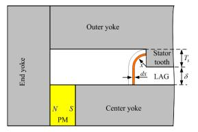
Figure 5. A circular-arc straight-line permeance model of tooth-to-center-yoke flux leakage.
