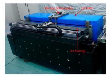
Figure 12. Prototype of RCDMC assembled in a horizontal ULF vibration exciter. Reproduced with permission from [19], IEEE, 2019.
