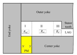
Figure 3. Magnetic flux leakage inside the RCDMC.
