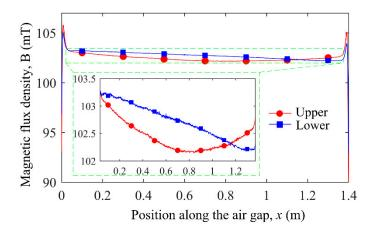
**Figure 13.** Measurement results of MFD along the upper and lower air gaps. Reproduced with permission from [19], IEEE, 2019.
