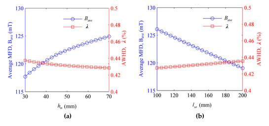
**Figure 10.** Average MFD and acceleration waveform harmonic distortion (AWHD) vs.: (a)  $h_{mi}$ ; (b)  $l_{se}$ .
