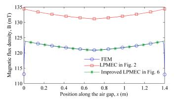
**Figure 9.** Magnetic flux density (MFD) distributions given by finite element method (FEM) and theoretical models.
