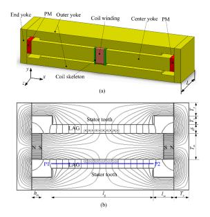
**Figure 1.** Schematic diagram of the rectangular closed double magnetic circuit (RCDMC): (a) 3D model; (b) 2D model, side view with magnetic flux lines. Reproduced with permission from [19], IEEE, 2019.
