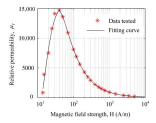
**Figure 7.** Polynomial fitting result of the H- $\mu_r$  curve of pure iron material.
