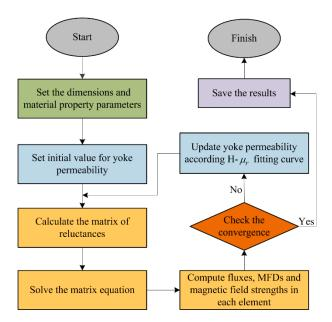
Figure 8. Procedures of the proposed iteration solving method.
