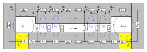
Figure 2. Lumped parameter magnetic equivalent circuit (LPMEC) model of the RCDMC.
