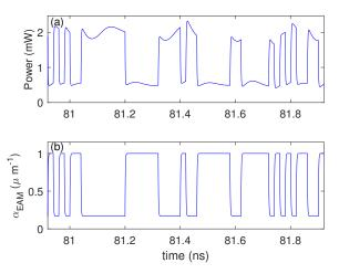
**Figure 7.** (color online) Time traces for digital, non-return-to-zero modulation of EAM VCSEL at 100 Gb/s. (a) Output power; (b)  $\alpha_{EAM}$ .
