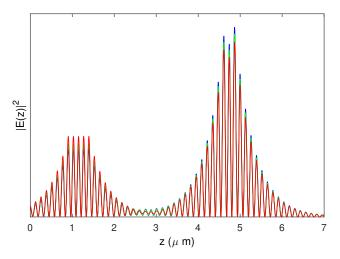
**Figure 1.** (color online) Optical power distributions along the EAM-VCSEL for  $d_{EAM} = 0.471 \,\mu\text{m}$  and  $\alpha_{EAM} = 1000 \,\text{cm}^{-1}$ . Blue, green and red curves are for  $\alpha_H^{VCL} = \alpha_H^{EAM} = 0$ ;  $\alpha_H^{VCL} = 2$ ,  $\alpha_H^{EAM} = 0$  and  $\alpha_H^{VCL} = 2$ ,  $\alpha_H^{EAM} = 1$ , respectively.
