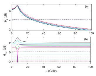
**Figure 5.** (color online) Same as Figure 4 but for the case of moderate coupling between EAM and VCSEL cavities ( $d_{EAM} = 0.5 \,\mu$ m). (a) and (b) correspond to modulation of injection current, i.e.,  $H_i(\nu)$  from Equation (21) and EAM losses  $\alpha_{EAM}$ , i.e.,  $H_{out}(\nu)$  from Equation (18), respectively.
