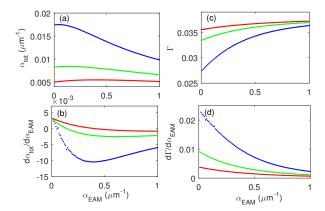
**Figure 3.** (color online) Dependence of (**a**) total absorption  $\alpha_{tot}$  of the EAM-VCSEL, (**b**) its derivative  $d\alpha_{tot}/d\alpha_{EAM}$ , (**c**) VCSEL cavity confinement factor  $\Gamma$  and (**d**) its derivative  $d\Gamma/d\alpha_{EAM}$  on the EAM absorption  $\alpha_{EAM}$ . Color coding for the three representative cases of different coupling strength between the EAM and VCSEL cavities are the same as for Figure 2.
