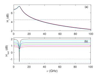
**Figure 6.** (color online) Same as Figure 4 but for the case of weak coupling between EAM and VCSEL cavities ( $d_{EAM} = 0.502 \,\mu\text{m}$ ). (a) and (b) correspond to modulation of injection current, i.e.,  $H_i(\nu)$  from Equation (21) and EAM losses  $\alpha_{EAM}$ , i.e.,  $H_{out}(\nu)$  from Equation (18), respectively.
