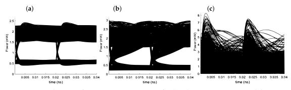
**Figure 8.** Eye diagrams of EAM-VCSEL output power for digital, non-return-to-zero modulation at 100 Gb/s. (a)  $d_{EAM} = 0.5025 \,\mu\text{m}$ ; (b)  $d_{EAM} = 0.501 \,\mu\text{m}$ ; (c)  $d_{EAM} = 0.504 \,\mu\text{m}$ .
