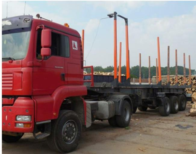
**Figure 1.** View of the truck stanchions with the displacement transducer before the timber was loaded.
