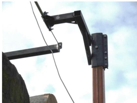
**Figure 3.** Displacement transducer mounted on the unloaded stanchion.
