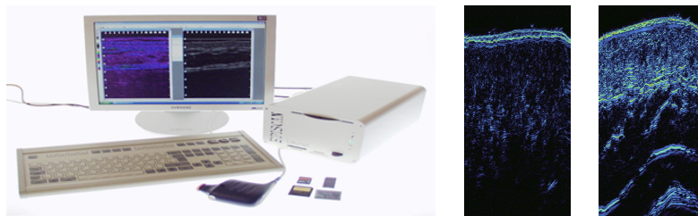
Figure 4. Episcan I-200 ultrasonic dermal scanner (left) and sample scans (right).
