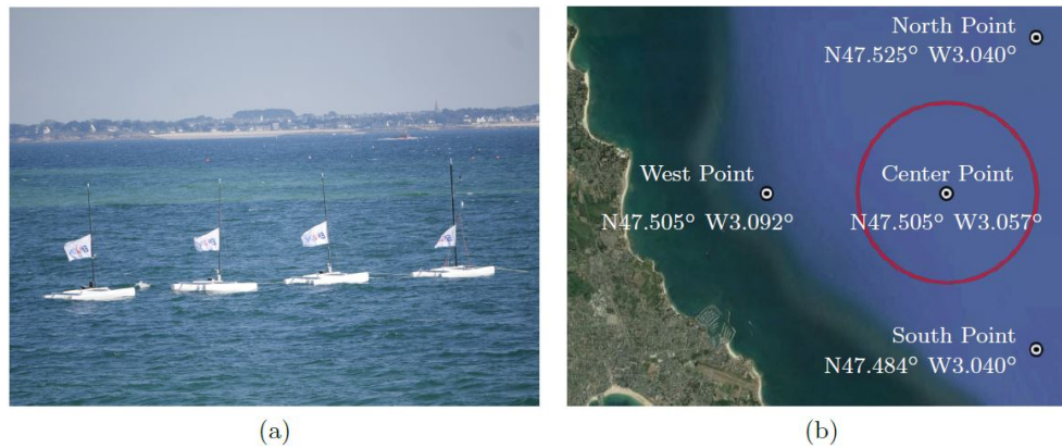
Figure 4. Fixed wind measurement points deployed. Picture (a) shows the 4 measurement platforms. Picture (b) shows position of the 4 measurement points during trials (white circle); the central one is always occupied by the platform fitted with the 3-anemometer mast (on the right in picture (a)); the external locations are occupied by the others fitted with single-anemometer masts. The red circle shows the limit of the area of measurement (0.7 NM radius).
